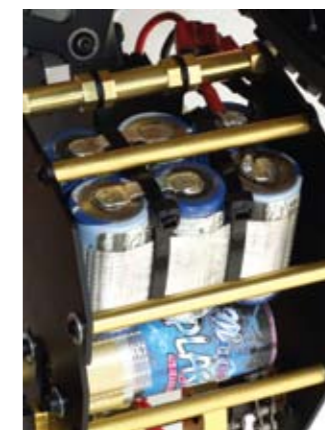
Unique battery layout. LiPo would weigh less, fit and perform better, especially 3S. A battery cover needs fabricating
