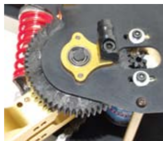
Primary drive is coarse. Layshaft mount has third leg for strength, and double as footpegs
