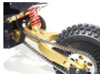
Alloy swing arm and chain final drive, GRP tyres were keen to get involved with the project
